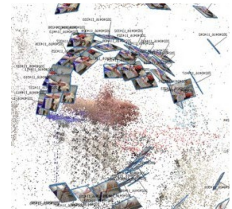
Fig. 2a: Photogrammetry-based 3D scan reconstruction process. The system captures and cleans overlapping hand images to generate a high-resolution mesh model used for orthosis design.
